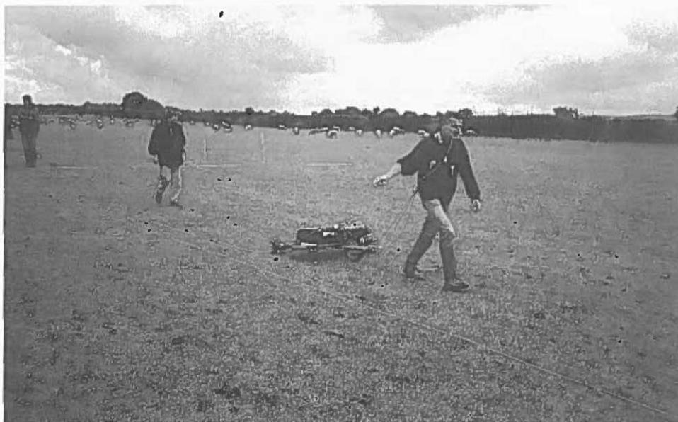
Fig. 3 – Albert Hesse using CNRS automated resistivity meter.
